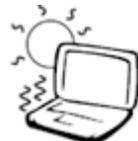
Do not expose to extreme temperatures above 50°C (122°F) or to direct sunlight. Do not block the fan vents (on the bottom, back, and sides of the laptop)!
